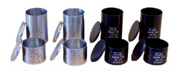
S.G. Cup Density cup is a stainless steel or anodized aluminium precision cup for determining the specific gravity or density of paints and similar products. The instrument consists of a cylindrical container and lid with a hole for the exhaust of excess liquid. Calibration Certificates are available and should be ordered at the time of purchase of the Cup.
